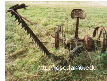
http://iqse.tamu.edu Circa 1885 Horse Drawn Sickle Type Hay Mower (driven by single horse or team)
